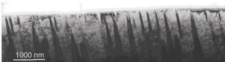
c/a/c/a 2-domain Structure (200 nm PZT 20/80 on SrTiO<sub>3</sub>)
